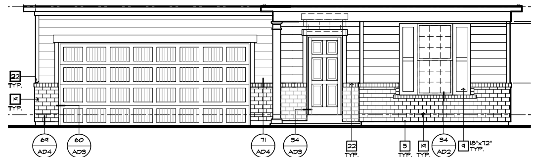
PARTIAL FRONT ELEVATION 'A' AT OPTIONAL 9'-1" PLT. HGT. W/ STONE OPT. SCALE 1/4"=1'-0" (22'x34') - 1/8"=1'-0" (11'x17')
