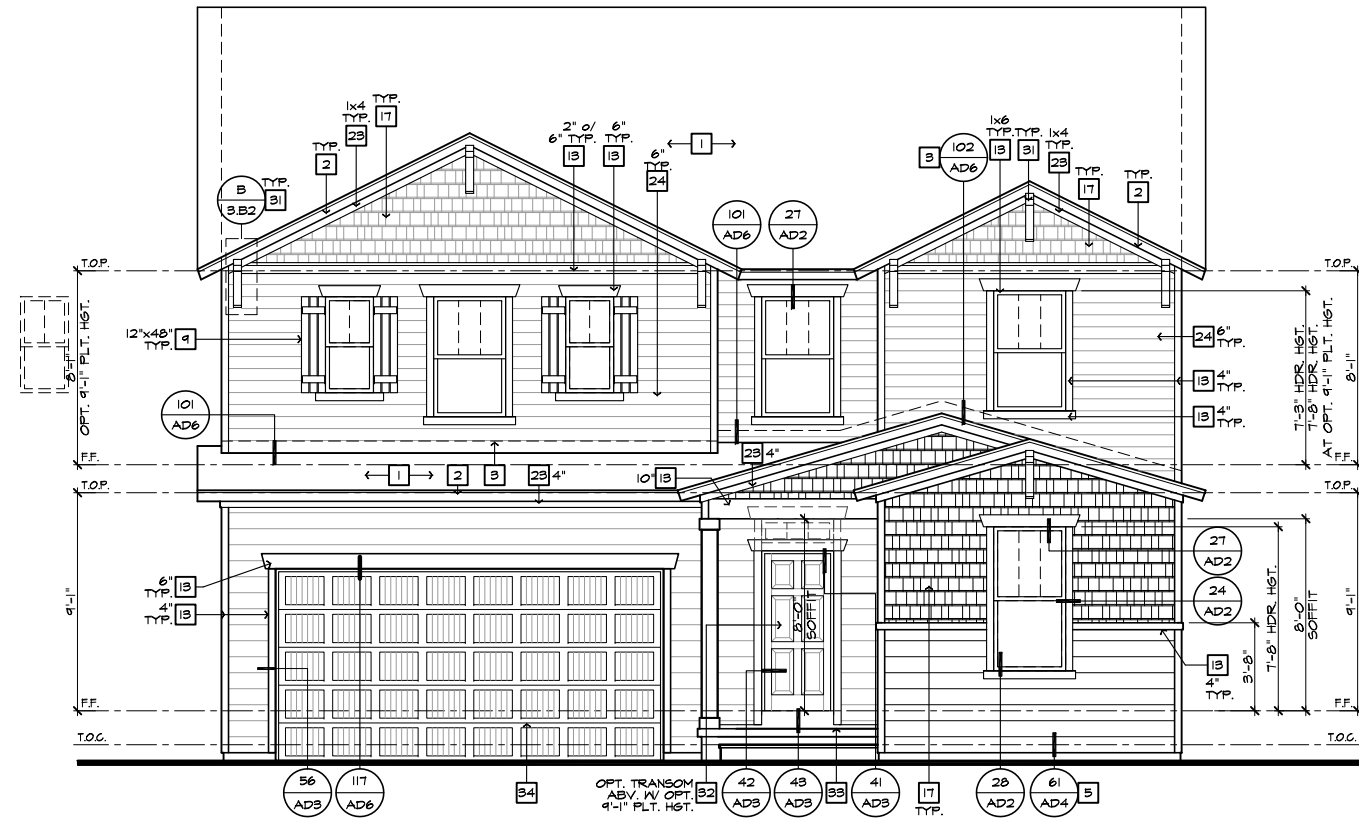
FRONT ELEVATION 'B' W/ CRAWL SPACE AT OPTIONAL 9'-1" PLT. HGT. SCALE 1/4"=1'-0" (22"X34") - 1/8"=1'-0" (11"X17")
