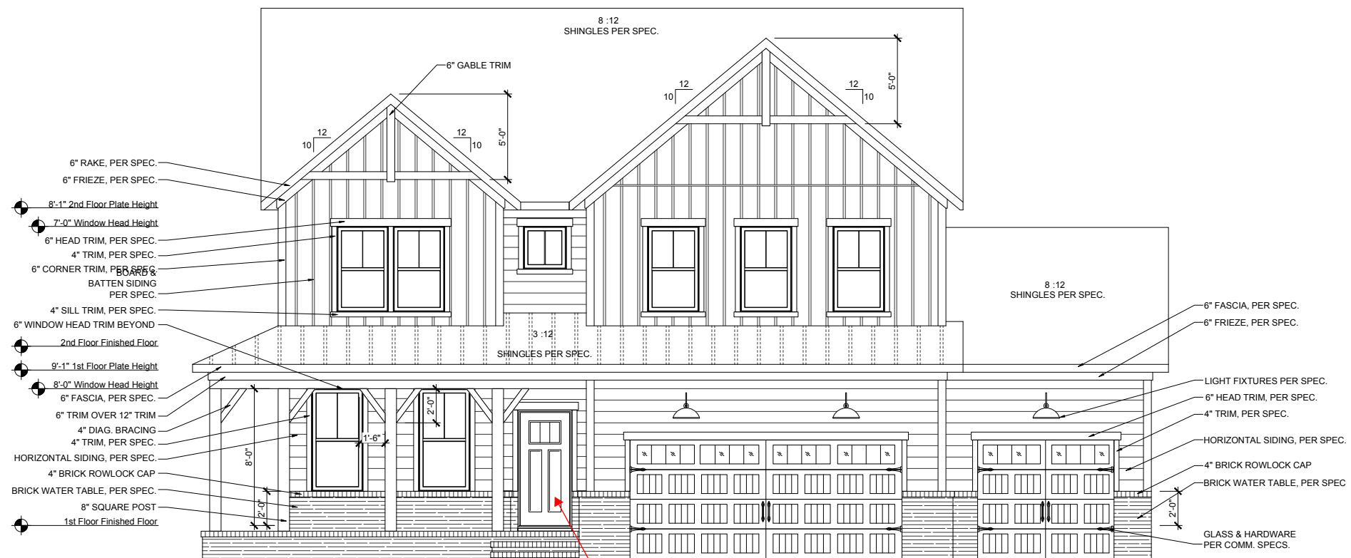
WILLOW OPT. 3RD CAR GARAGE FRONT ELEVATION - E SCALE: 1/8"=1'-0" (11"x17" SHEET SIZE) SCALE: 1/4"=1'-0" (22"x34" SHEET SIZE)
