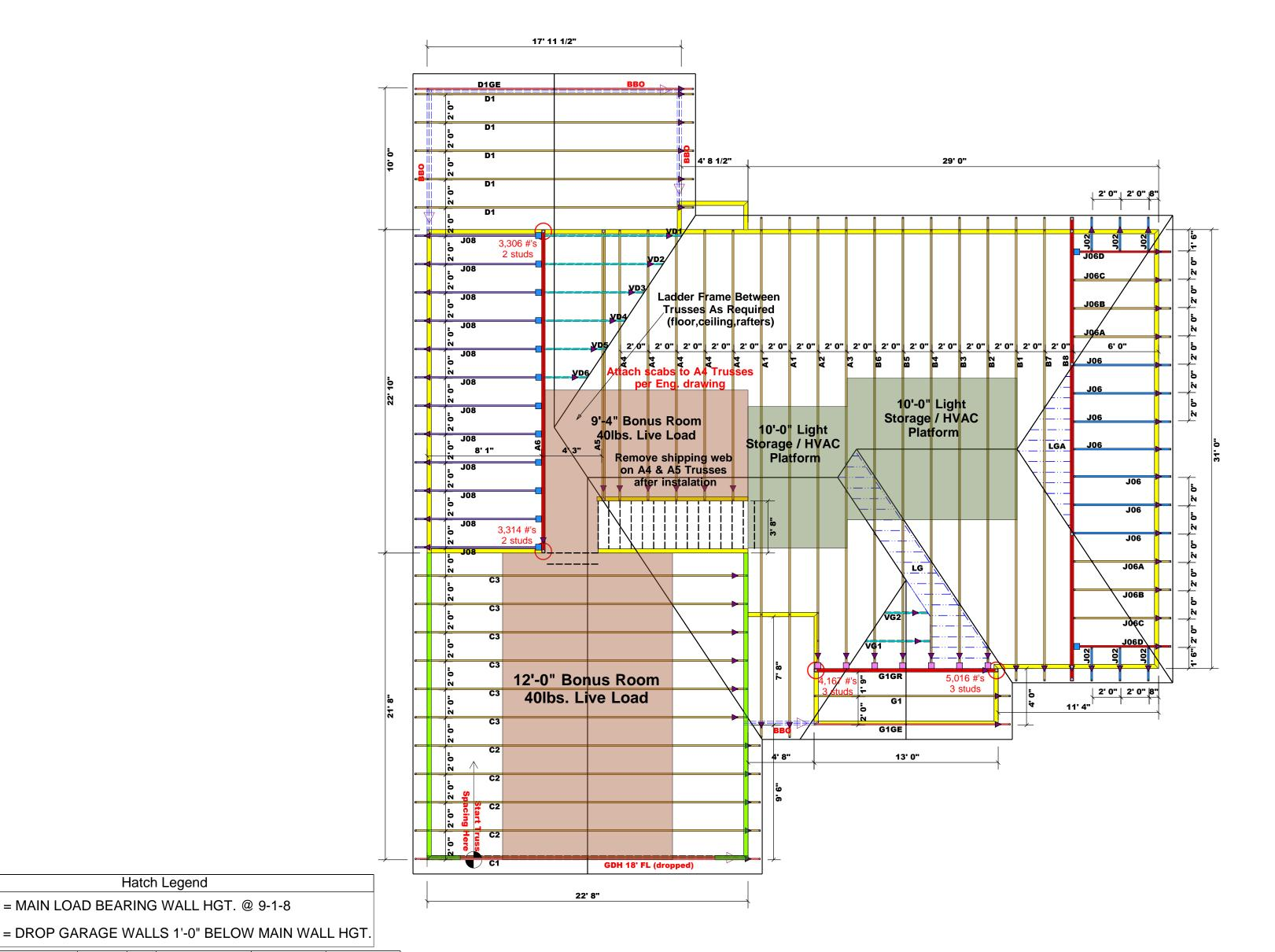
▲= Denotes Left End of Truss (Reference Engineered Truss Drawing)
