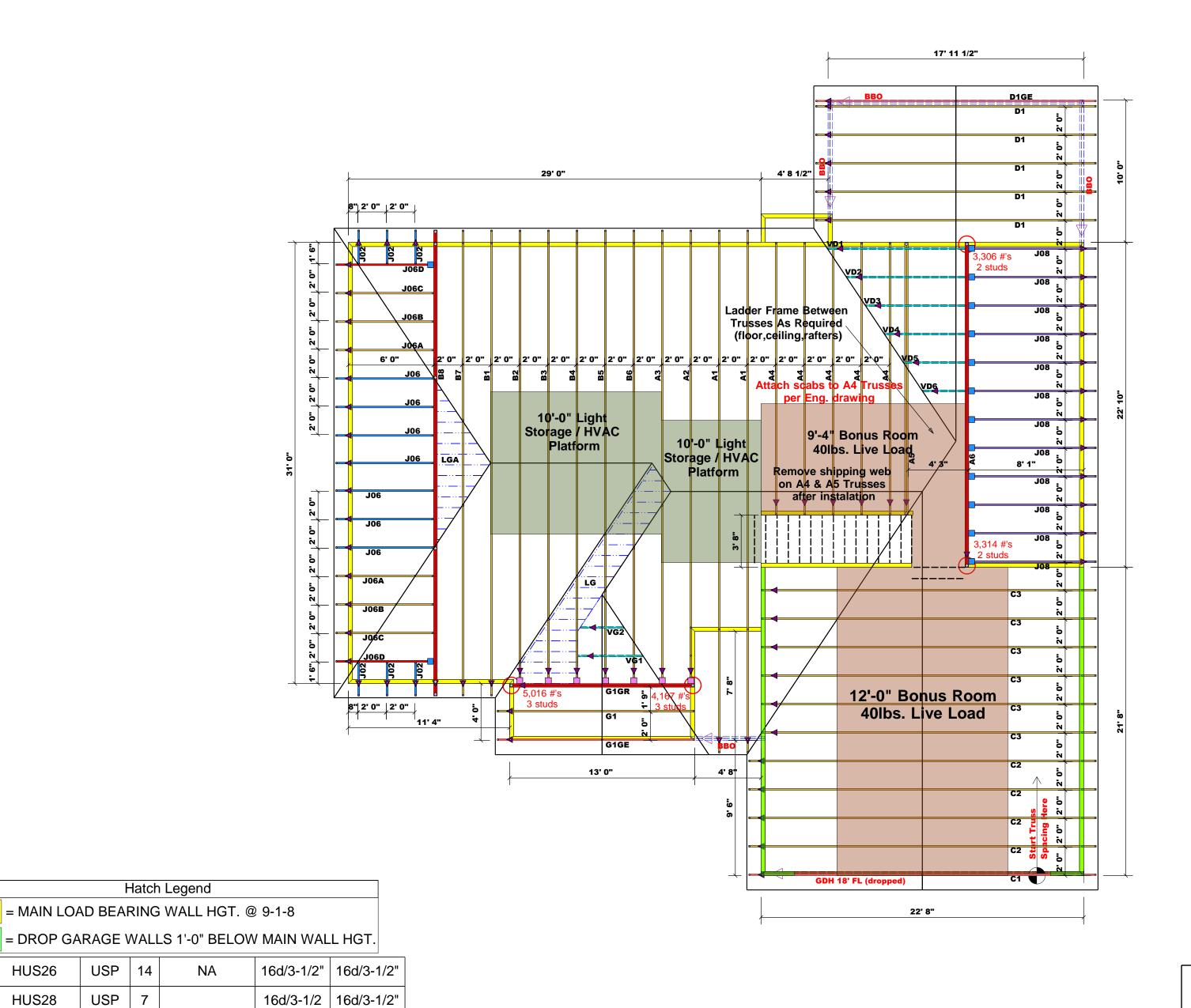
**Truss Placement Plan**
