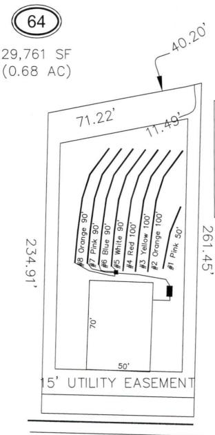
\*House footprint to be field staked by surveyor and system verified prior to any construction
