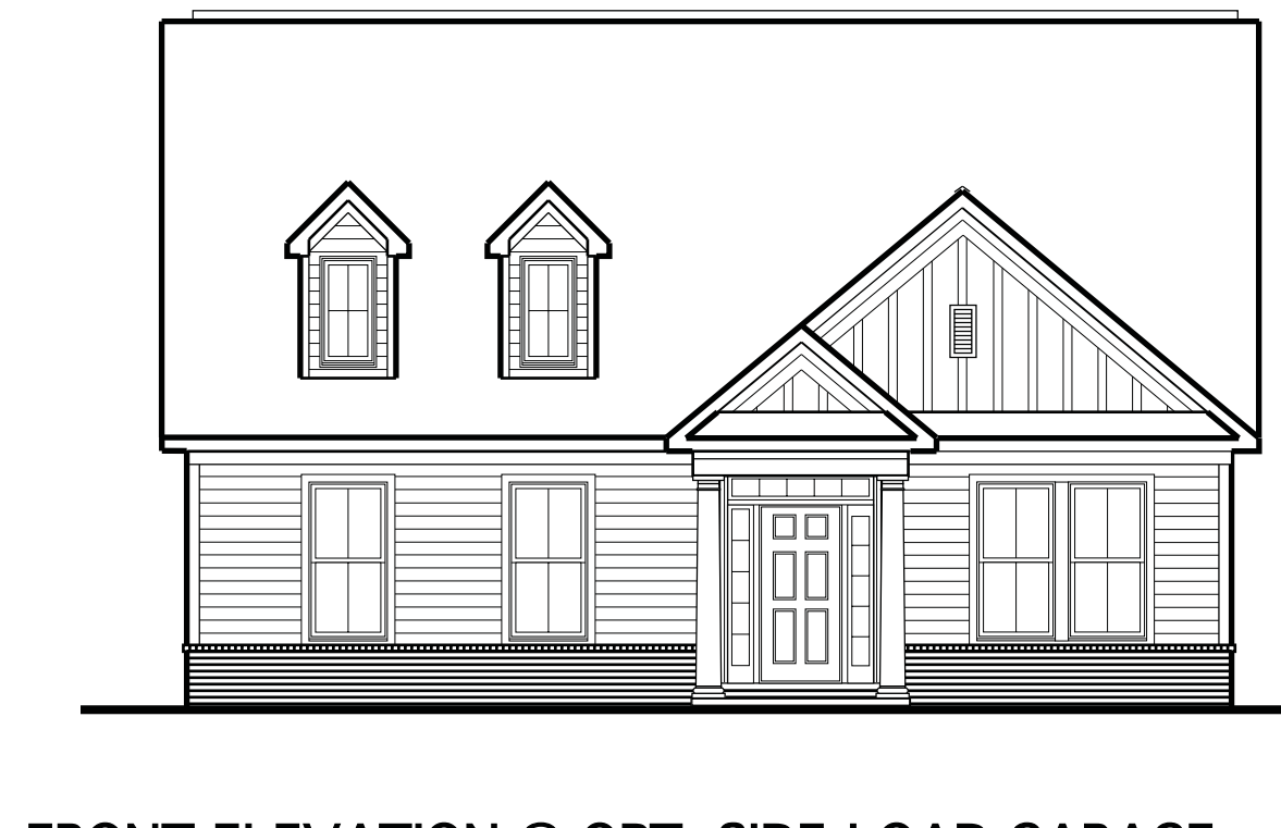
FRONT ELEVATION @ OPT. SIDE-LOAD GARAGE SCALE: 1/8" = 1'-0"
