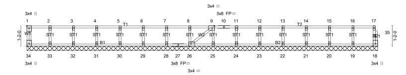
20-0-14 Plate Offsets (X,Y)-- [1:Edge,0-1-8], [9:0-1-8,Edge], [26:0-1-8,Edge], [34:Edge,0-1-8] LOADING (psf) SPACING-DEFL PLATES **GRIP** 2-0-0 CSI. in (loc) I/defl I/d **TCLL** 40.0 Plate Grip DOL 1.00 TC 0.06 Vert(LL) n/a n/a 999 MT20 244/190 TCDL 10.0 Lumber DOL 1.00 вс 0.01 Vert(CT) n/a n/a 999 YES WB 0.03 0.00 **BCLL** 0.0 Rep Stress Incr Horz(CT) 18 n/a n/a BCDL Code IRC2021/TPI2014 Weight: 86 lb FT = 20%F, 11%E Matrix-SH
