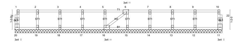
12-3-4 12-3-4 Plate Offsets (X,Y)-- [6:0-1-8,Edge], [16:0-1-8,Edge], [20:Edge,0-1-8] LOADING (psf) SPACING-CSI. DEFL. PLATES **GRIP** 2-0-0 in (loc) I/defl I/d **TCLL** 40.0 Plate Grip DOL 1.00 TC 0.08 Vert(LL) n/a n/a 999 MT20 244/190 TCDL 10.0 Lumber DOL 1.00 вс 0.01 Vert(CT) n/a n/a 999 **BCLL** YES WB 0.04 0.00 0.0 Rep Stress Incr Horz(CT) 11 n/a n/a BCDL Code IRC2021/TPI2014 Matrix-SH Weight: 54 lb FT = 20%F, 11%E
