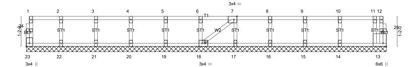
13-9-4 Plate Offsets (X,Y)-- [7:0-1-8,Edge], [13:Edge,0-1-8], [18:0-1-8,Edge], [23:Edge,0-1-8] LOADING (psf) SPACING-DEFL PLATES **GRIP** 2-0-0 CSI. in (loc) I/defl I/d **TCLL** 40.0 Plate Grip DOL 1.00 TC 0.06 Vert(LL) n/a n/a 999 MT20 244/190 TCDL 10.0 Lumber DOL 1.00 вс 0.01 Vert(CT) n/a n/a 999 **BCLL** YES WB 0.03 0.00 0.0 Rep Stress Incr Horz(CT) 13 n/a n/a BCDL Code IRC2021/TPI2014 Weight: 61 lb FT = 20%F, 11%E Matrix-SH
