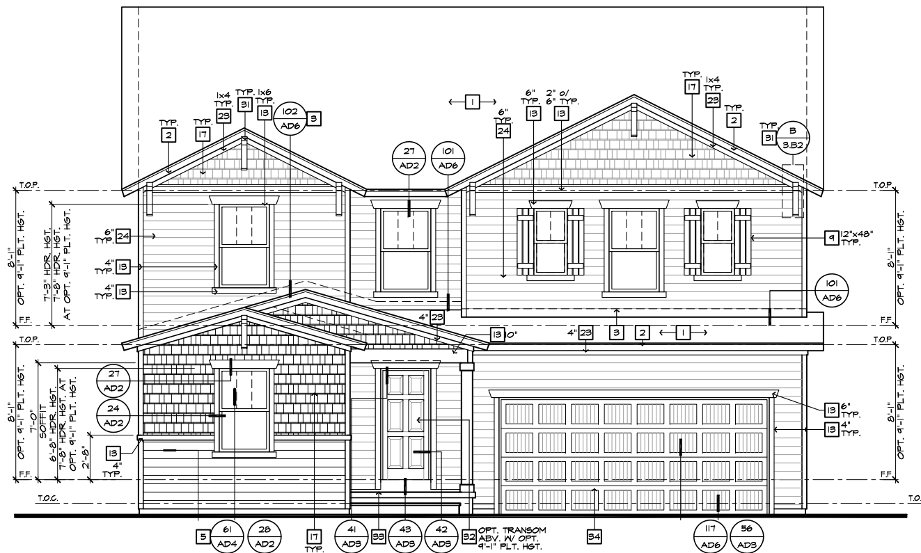
FRONT ELEVATION 'B' W/ CRAWL SPACE
