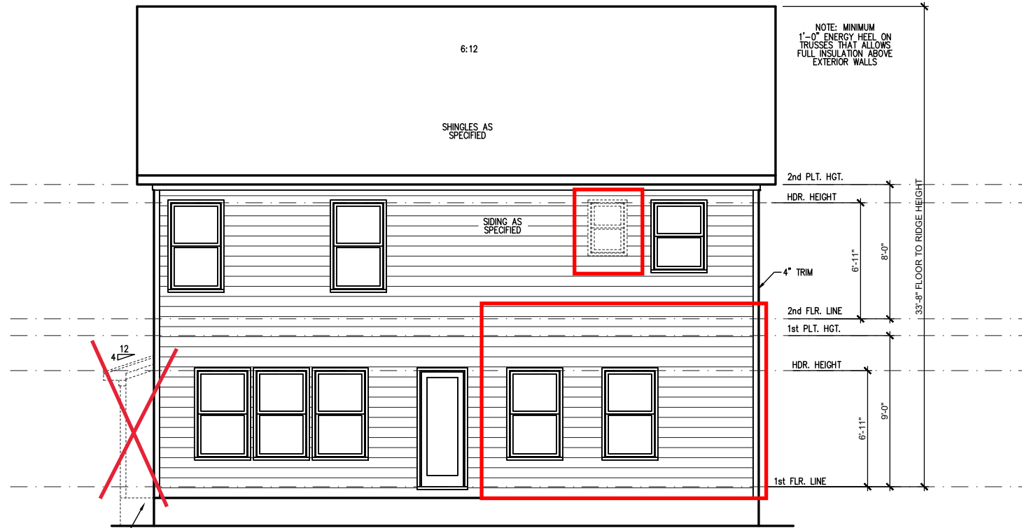
REAR ELEVATION 'CRAFTSMAN' (CRAWL/STEM WALL) SCALE: 1/4" = 1'-0" ON 22x34, 1/8" = 1'-0" ON 11x17 SEE FOUNDATION PAGES FOR FOUNDATION TYPE
