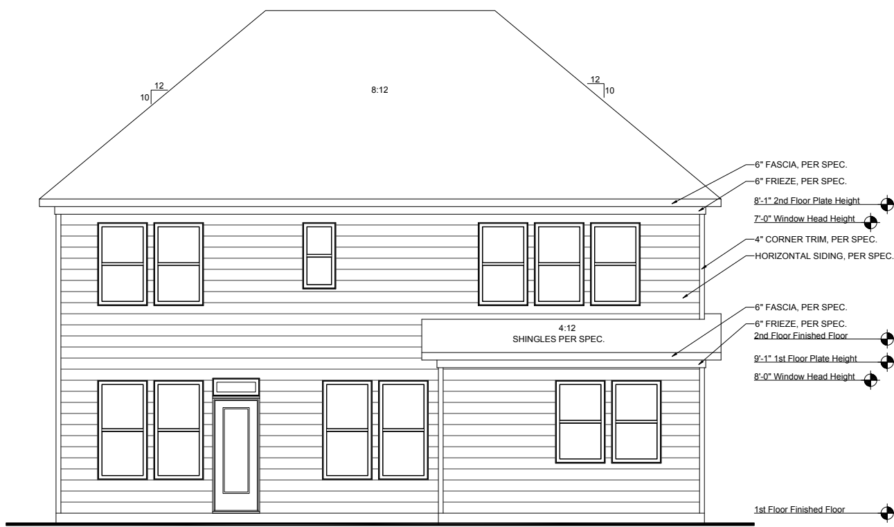
OPT. GUEST SUITE REAR ELEVATION SCALE: 1/8"=1'-0" (11"X17" SHEET SIZE) SCALE: 1/4"=1'-0" (22"X34" SHEET SIZE)
