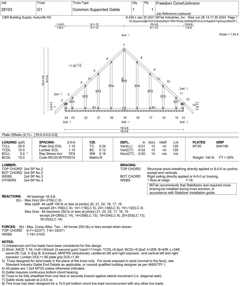
9) \* This truss has been designed for a live load of 20.0psf on the bottom chord in all areas with a clearance greater than 6-0-0 between the bottom chord and any other members, with BCDL = 10.0psf.
