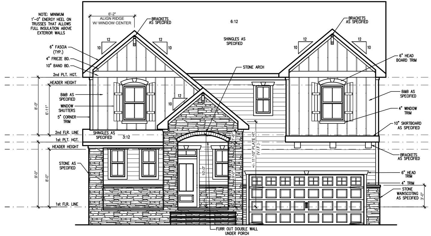
FRONT ELEVATION 'FRENCH COUNTRY' (CRAWL/STEM WALL) SCALE: 1/4" = 1'-0" ON 22x34, 1/8" = 1'-0" ON 11x17 *SEE FOUNDATION PAGES FOR FOUNDATION TYPE
