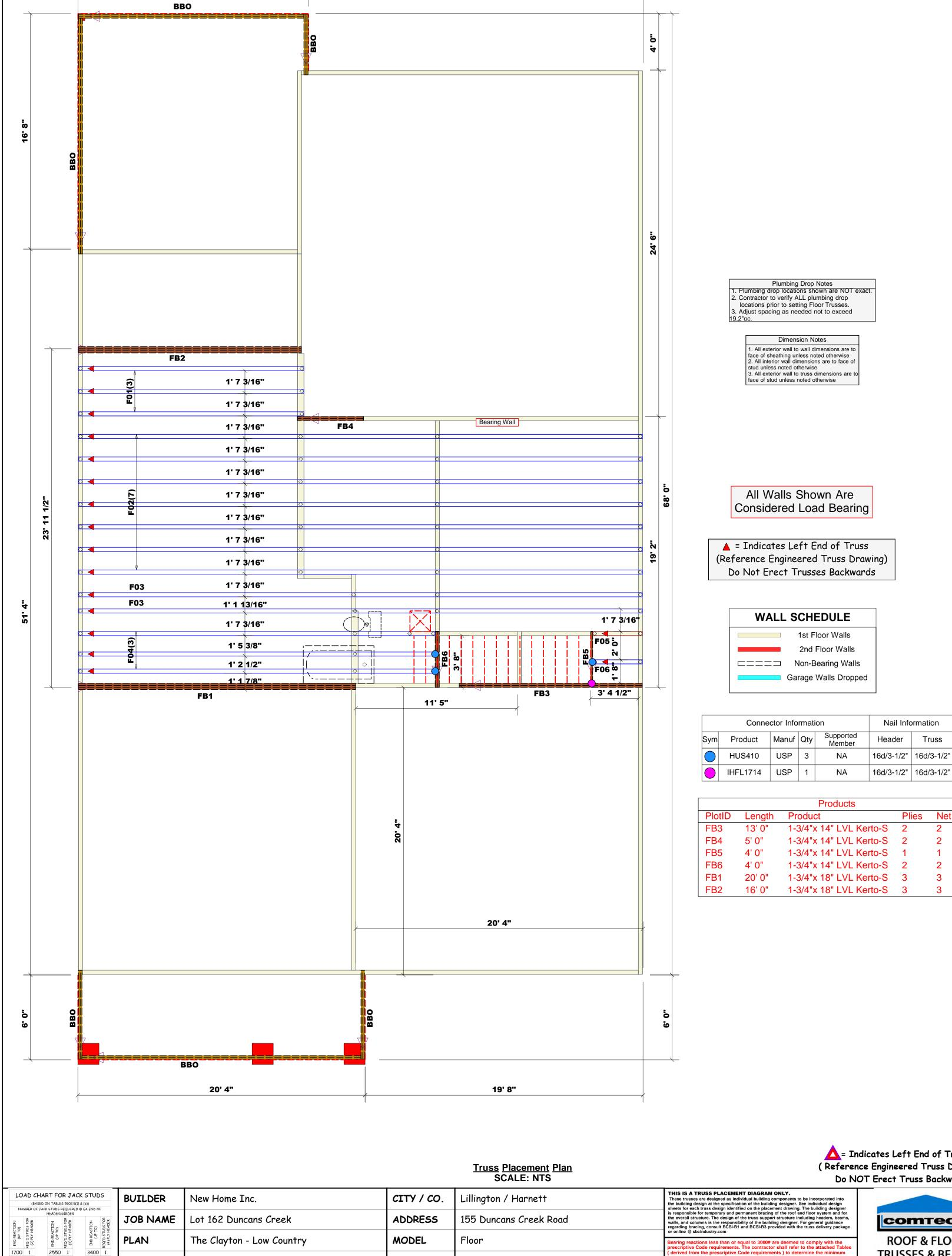
= Indicates Left End of Truss (Reference Engineered Truss Drawing) Do NOT Erect Truss Backwards
