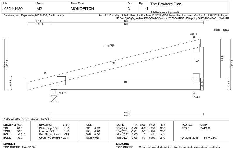
TOP CHORD 2x4 SP No.1 BOT CHORD 2x6 SP No.1 WEBS 2x6 SP No.1 TOP CHORD BOT CHORD Structural wood sheathing directly applied, except end verticals. Rigid ceiling directly applied.
