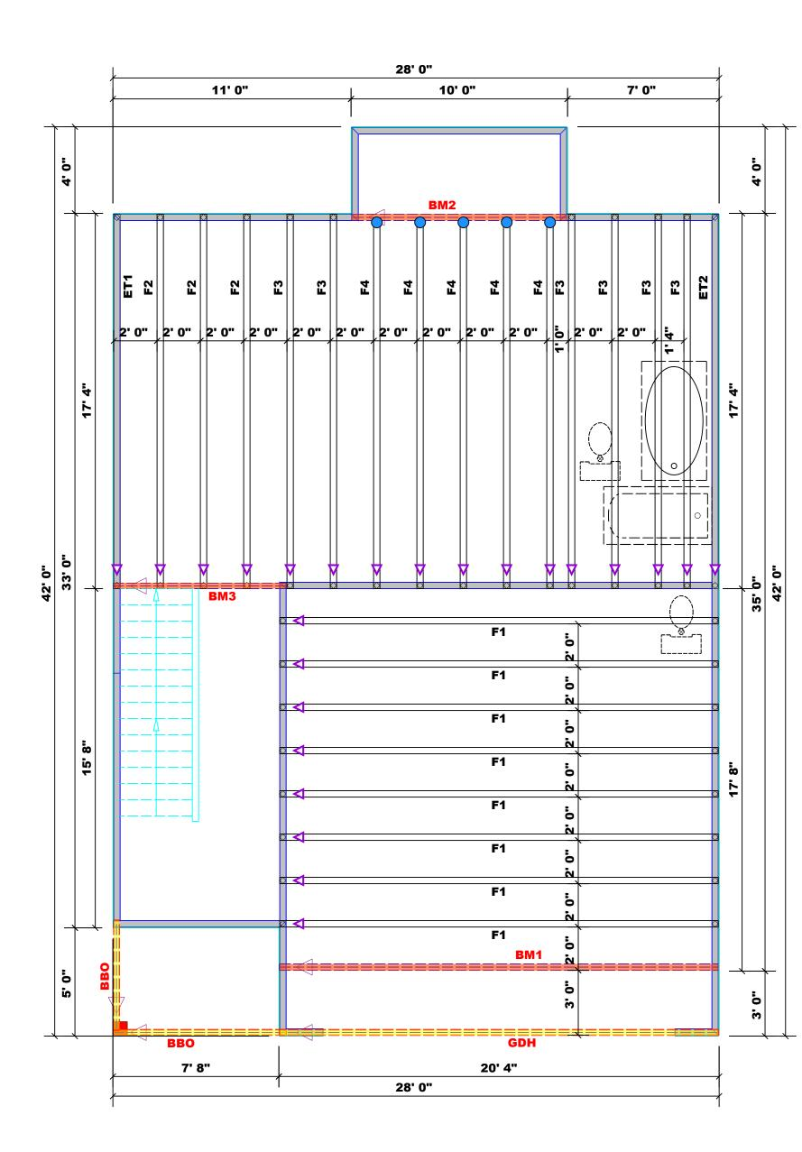
= Indicates Left End of Truss (Reference Engineered Truss Drawing) Do NOT Erect Truss Backwards
