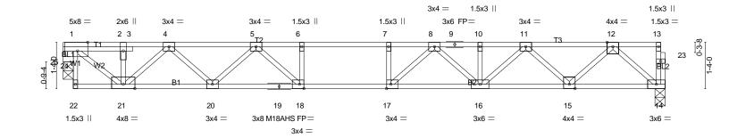
17-3-8 Plate Offsets (X,Y)-- [1:0-3-8,Edge], [17:0-1-8,Edge], [18:0-1-8,Edge] SPACING-DEFL. **PLATES GRIP** LOADING (psf) in (loc) I/defI L/d **TCLL** 40.0 Plate Grip DOL 1.00 TC 0.76 Vert(LL) -0.26 16-17 >796 480 MT20 244/190 TCDL Lumber DOL ВС 0.88 Vert(CT) -0.34 16-17 10.0 1.00 >599 360 M18AHS 186/179 WB 0.63 0.03 **BCLL** 0.0 Rep Stress Incr YES Horz(CT) 14 n/a n/a Code IRC2015/TPI2014 BCDI 5.0 Matrix-S Weight: 92 lb FT = 20%F, 11%E
