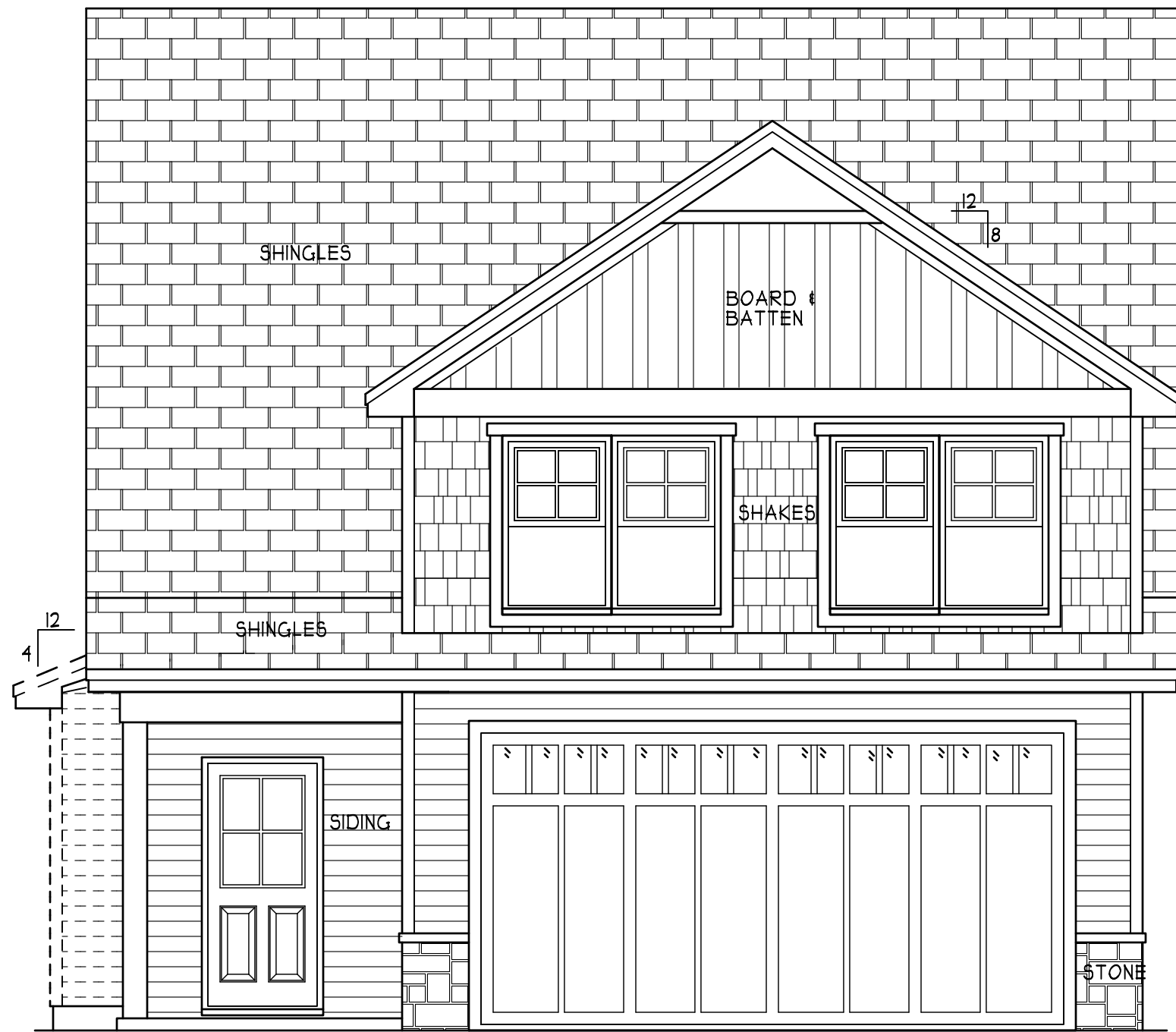
OPT ELEVATION SCALE 1/4" = 1'-0"
