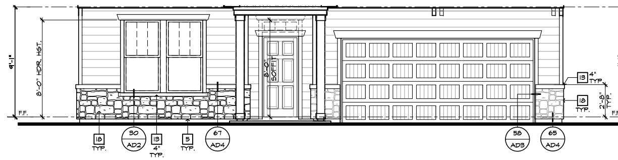
PARTIAL FRONT ELEVATION 'B' AT OPTIONAL 9'-1" PLT. HGT. W/ STONE OPT.
