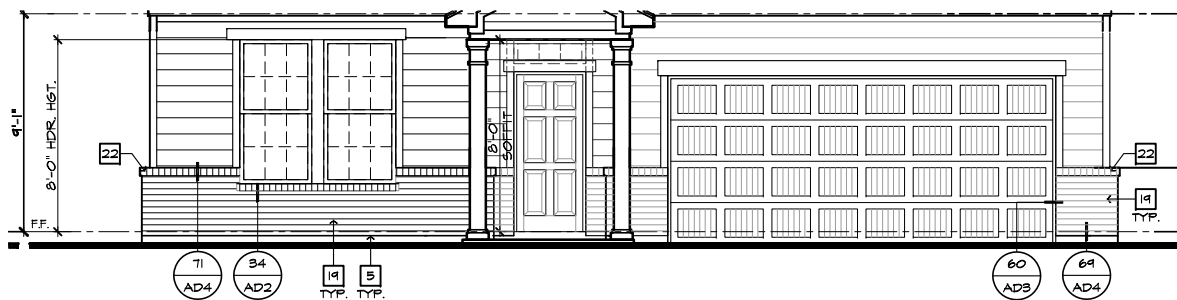
PARTIAL FRONT ELEVATION 'A' AT OPTIONAL 9'-1" PLT. HGT. W/ BRICK OPT.
