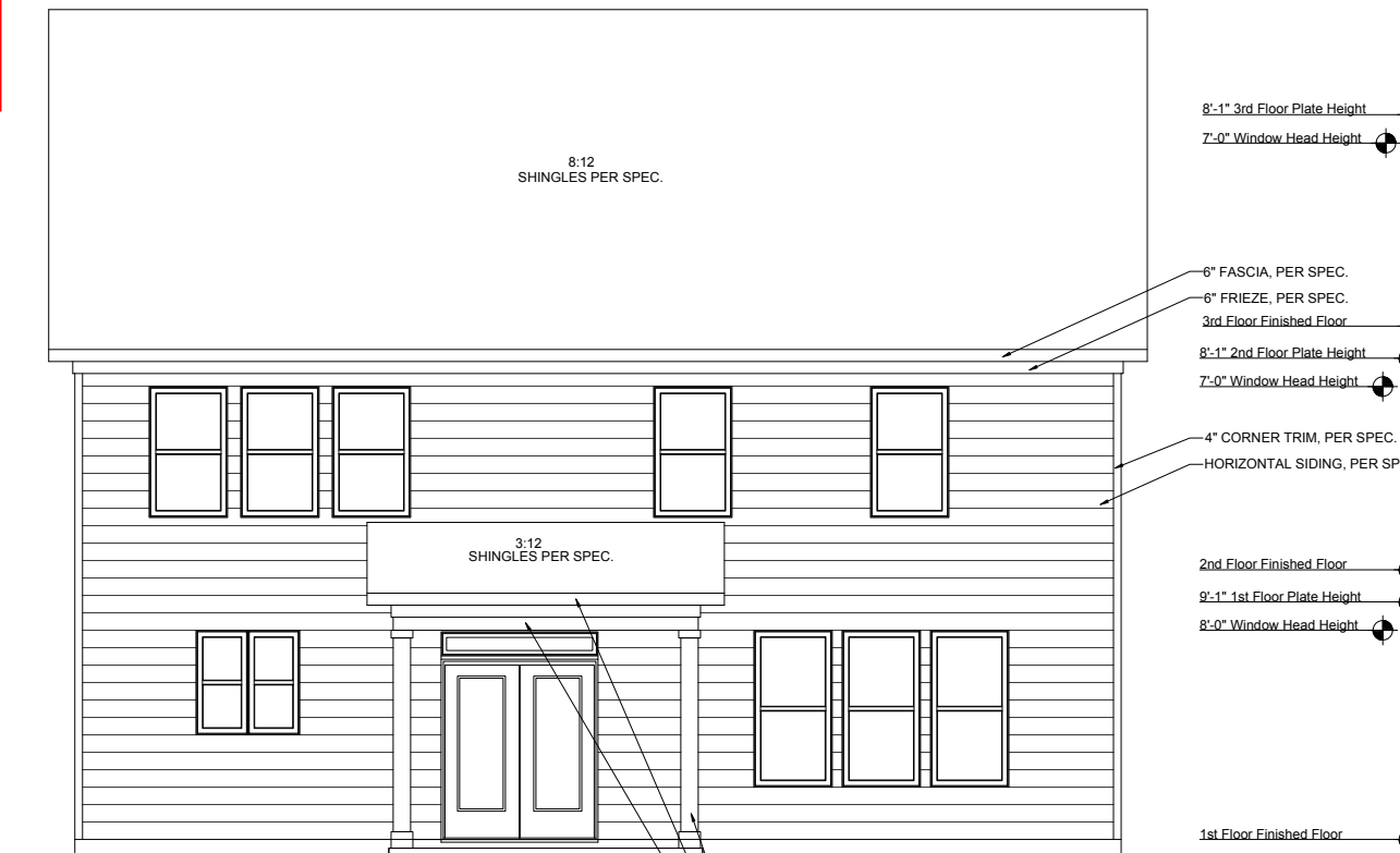
COVERED PORCH REAR ELEVATION
