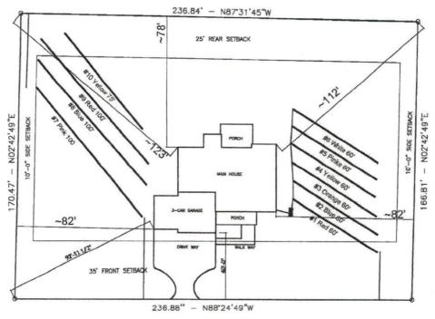
System: Gravity to serial distribution
