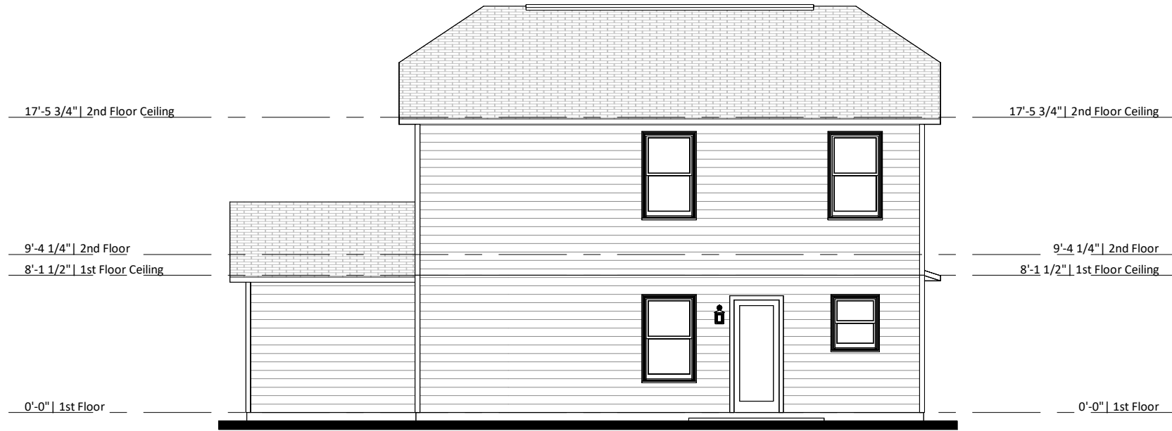
② Rear Elevation - Elev B - 2 Car Garage 1/8" = 1'-0"
