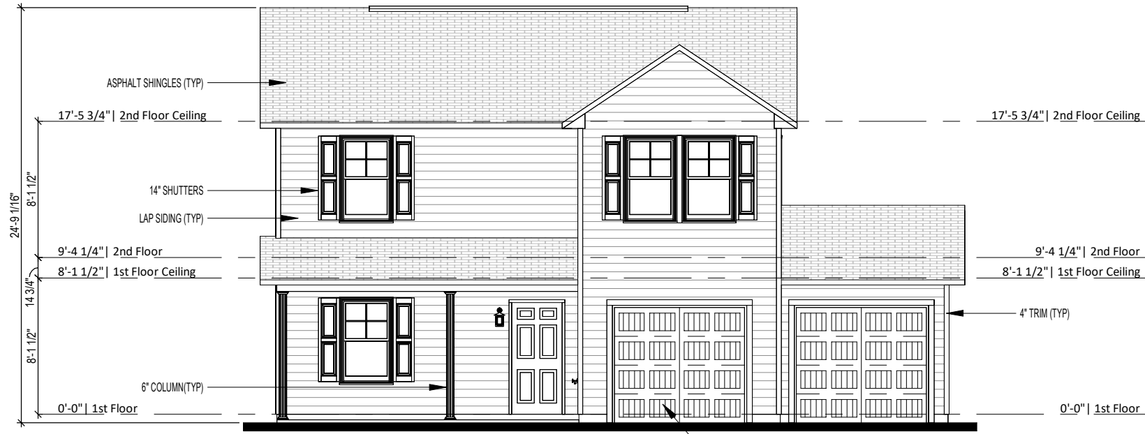
① Front Elevation - Elev A - 2 Car Garage 1/8" = 1'-0"
