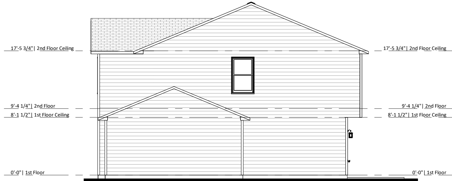
① Right Elevation - Elev A - 2 Car Garage 1/8" = 1'-0"
