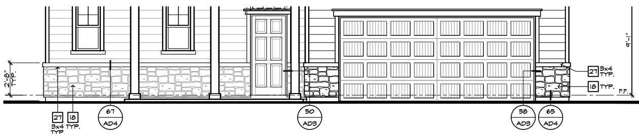
PARTIAL FRONT ELEVATION 'C' W/ MASONRY OPTION AT 9'-0" PLT. HGT. SCALE 1/4"=1'-0" (22"X34") - 1/8"=1'-0" (11"X17")
