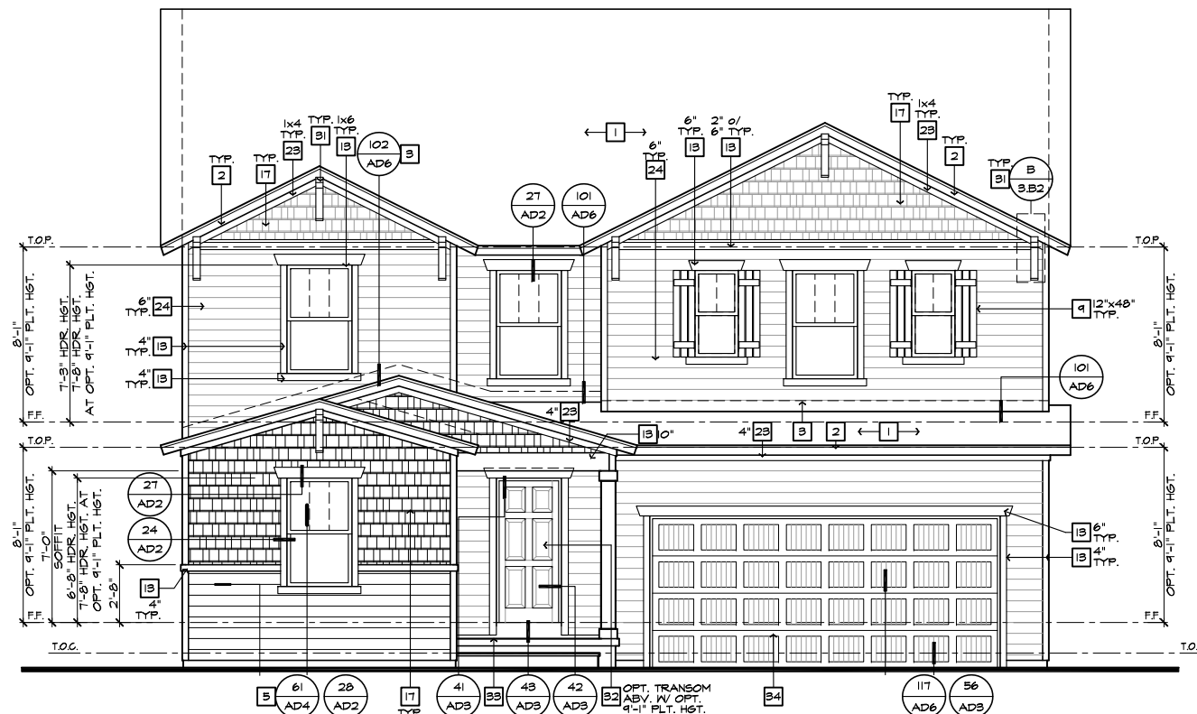
FRONT ELEVATION 'B' W/ CRAWL SPACE
