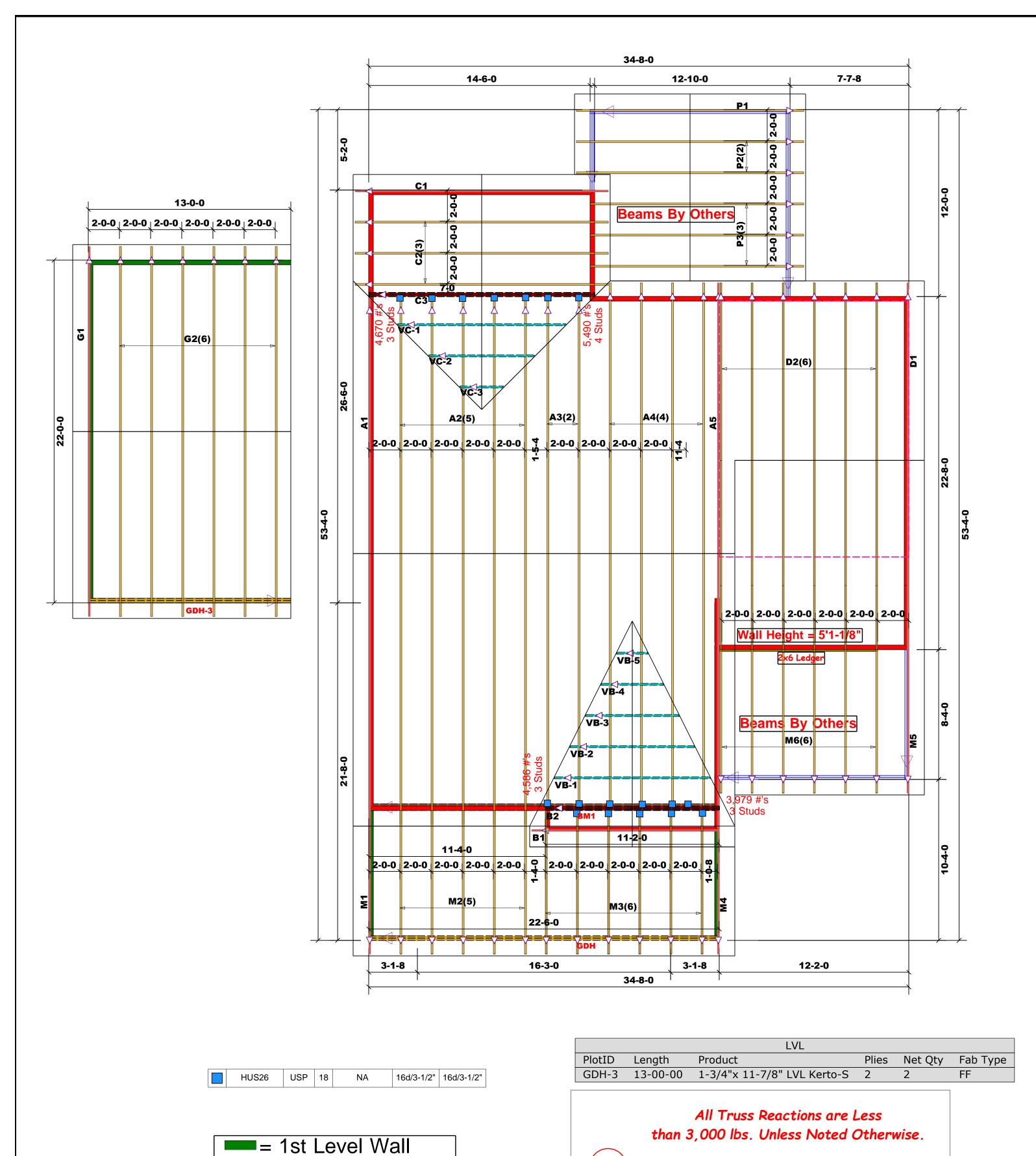
Truss Placement Plan SCALE: 1/4"=1'
