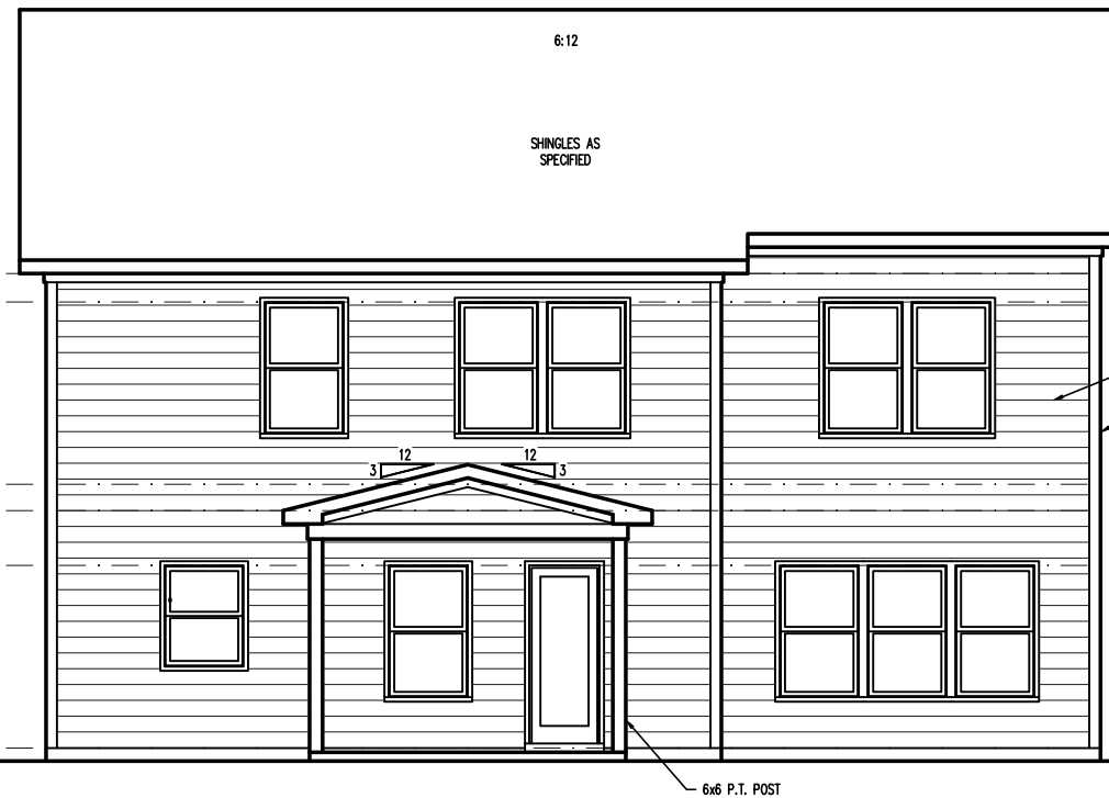
COVERED PORCH REAR ELEVATION (SLAB)
