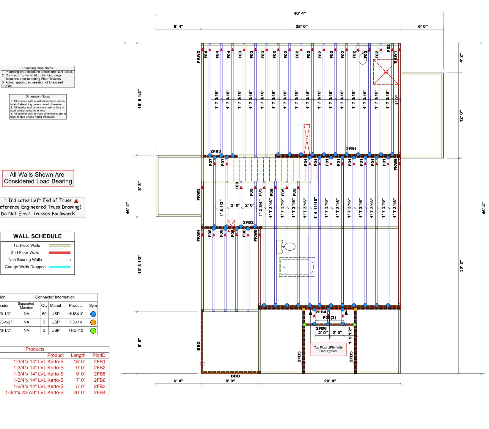
Considered Load Bearing = Indicates Left End of Truss 🔺 (Reference Engineered Truss Drawing) Do Not Erect Trusses Backwards
