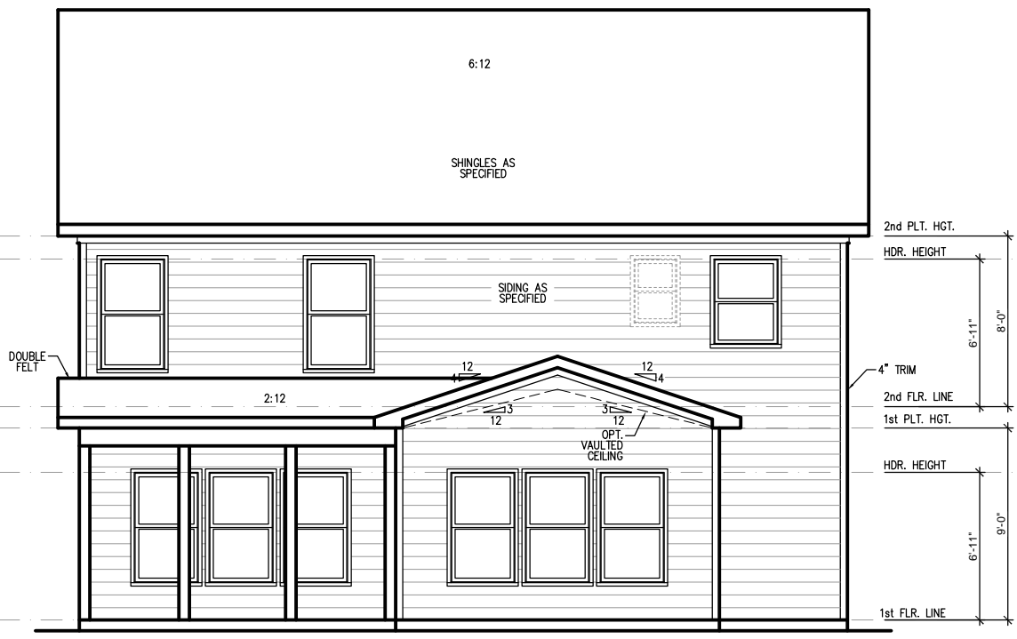
EXTENDED CAFE W/ COVERED PORCH REAR ELEVATION SCALE: 1/8"=1'-0" ON 11x17, 1/4"=1'-0" ON 22x34
