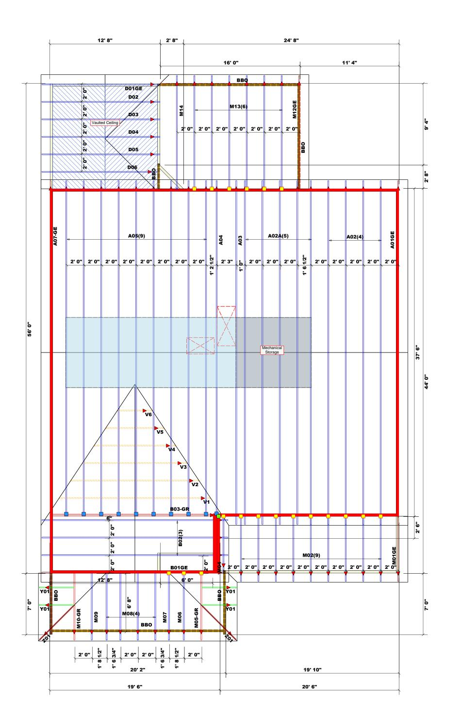
= Indicates Left End of Truss (Reference Engineered Truss Drawing) Do NOT Erect Truss Backwards
