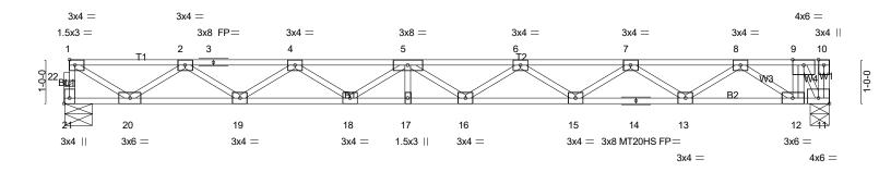
16-8-4 17-4-12 0-8-8 16-8-4 Plate Offsets (X,Y)-- [11:Edge,0-1-8], [21:Edge,0-1-8] LOADING (psf) SPACING-DEFL **PLATES GRIP** 1-4-0 CSI. in (loc) I/defl I/d **TCLL** 40.0 Plate Grip DOL 1.00 TC 0.44 Vert(LL) -0.2416 >868 480 MT20 244/190 TCDL 10.0 Lumber DOL 1.00 вс 0.71 Vert(CT) -0.36 16 >568 360 MT20HS 187/143 WB 0.50 0.06 **BCLL** 0.0 Rep Stress Incr NO Horz(CT) 11 n/a n/a BCDL Code IRC2021/TPI2014 Weight: 88 lb FT = 20%F, 11%E Matrix-SH
