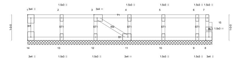
7-3-0 Plate Offsets (X,Y)-- [1:Edge,0-1-8], [3:0-1-8,Edge], [11:0-1-8,Edge], [14:Edge,0-1-8] LOADING (psf) SPACING-DEFL PLATES **GRIP** 2-0-0 CSI. in (loc) I/defl I/d **TCLL** 40.0 Plate Grip DOL 1.00 TC 0.06 Vert(LL) n/a n/a 999 MT20 244/190 TCDL 10.0 Lumber DOL 1.00 вс 0.01 Vert(CT) n/a n/a 999 **BCLL** YES WB 0.03 -0.00 0.0 Rep Stress Incr Horz(CT) 8 n/a n/a BCDL Code IRC2021/TPI2014 Weight: 33 lb FT = 20%F, 11%E Matrix-P
