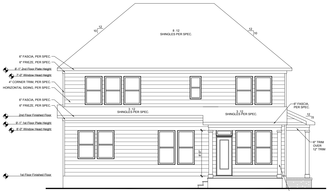
OPT. EXTENDED FAMILY W/ OPT. COVERED PORCH REAR ELEVATION SCALE: 1/8"=1'-0" (11"X17" SHEET SIZE) SCALE: 1/4"=1'-0" (22"X34" SHEET SIZE)
