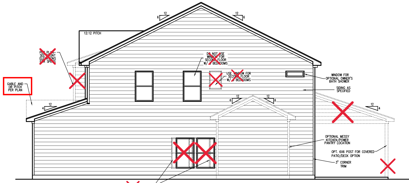
Patio Only No Cov. Porch RIGHT ELEVATION (SLAB) SCALE: 1/4" = 1'-0" ON 22x34, 1/8" = 1'-0" ON 11x17
