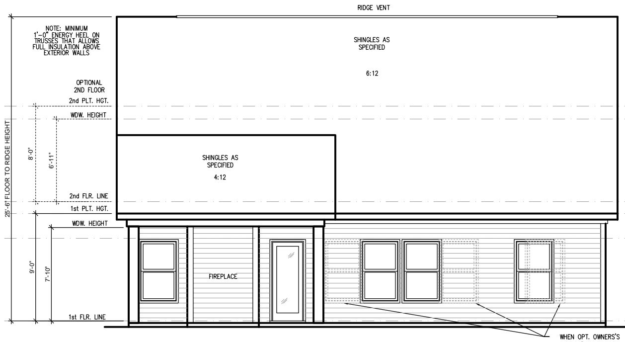
OPT. EXT. COVERED PORCH W/FIREPLACE REAR ELEVATION SCALE: 1/8"=1'-0" ON 11x17, 1/4"=1'-0" ON 22x34
