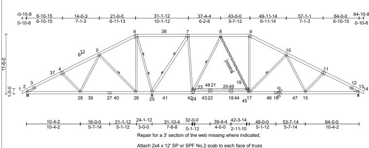
as shown with 2 rows of 10d (.131" x 3") nails spaced 4" oc [2:0-3-2,0-0-8], [4:0-4-0,0-4-8], [6:0-3-4,0-3-8], [7:0-3-12,0-5-0], [11:0-4-0,0-4-8], [13:Edge,0-2-10], [24:0-4-0,0-4-8]
