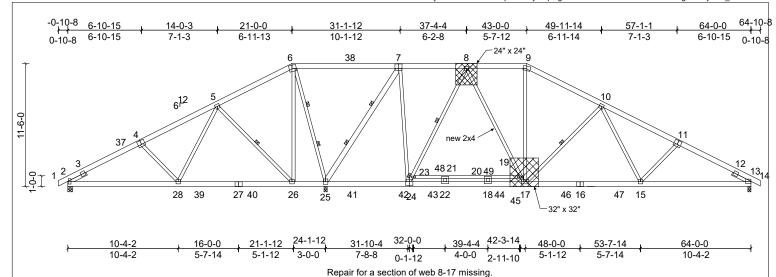
Cut and fit tight a new 2x4 SP or SPF No.2 web, and attach 1/2" Plywood or 7/16" OSB (APA Rated Sheathing Exposure 1) gussets
