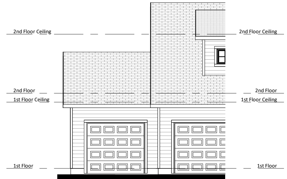
3 Opt. 3rd Car Garage - Front Elevation 1/8" = 1'-0"
