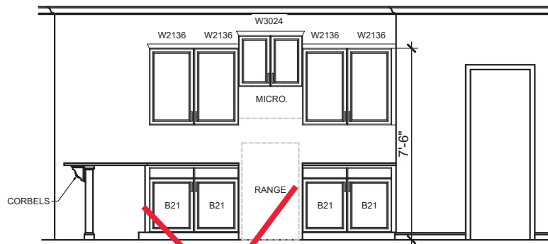
A - CABINET ELEVATION
