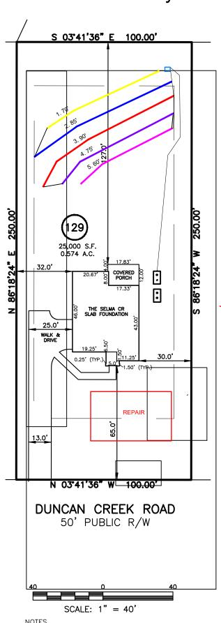
Adams Soil Consulting 919—414—6761 INITIAL: Lines 1-5 (380') Accepted Status Pump to Serial REPAIR: PPBPS Pressure Manifold
