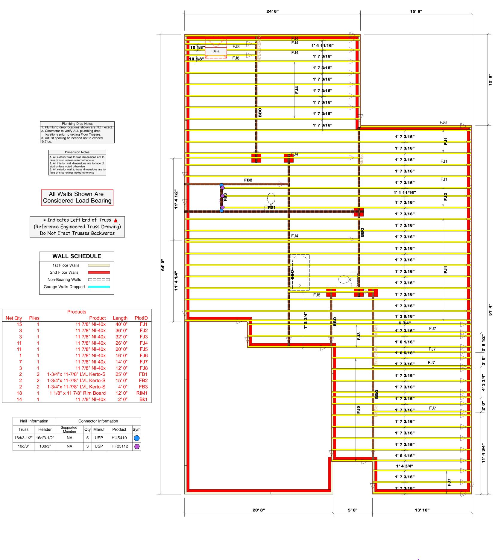
Truss Placement Plan **SCALE: NTS**
