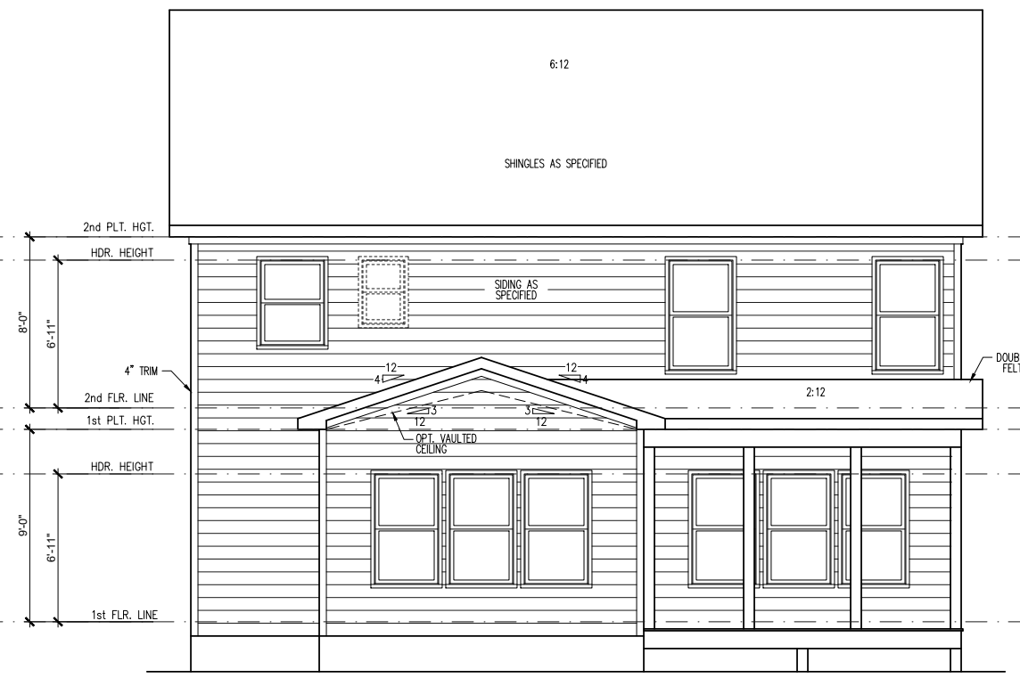
EXTENDED CAFE W/ COVERED PORCH REAR ELEVATION (CRAWL/ STEM WALL) SCALE: 1/8"=1'-0" ON 11x17, 1/4"=1'-0" ON 22x34 SEE FOUNDATION PAGES FOR FOUNDATION TYPE
