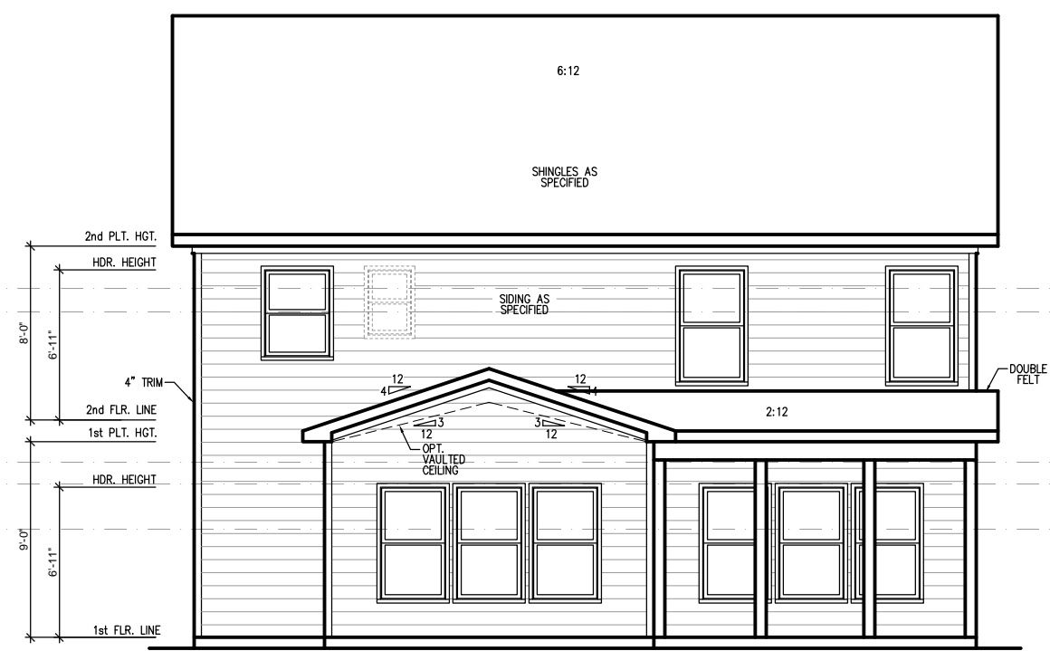
EXTENDED CAFE W/ COVERED PORCH REAR ELEVATION SCALE: 1/8"=1'-0" ON 11x17, 1/4"=1'-0" ON 22x34
