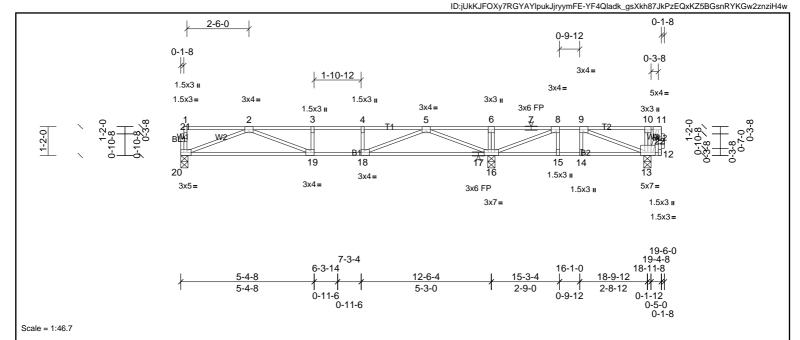
Plate Offsets (X, Y): [8:0-1-8,Edge], [9:0-1-8,Edge], [11:0-1-8,Edge], [18:0-1-8,Edge], [19:0-1-8,Edge], [20:0-2-0,Edge]
