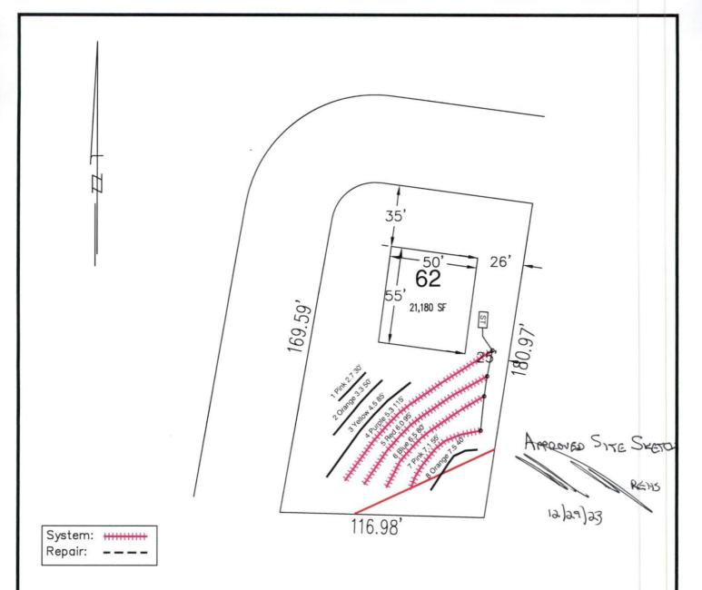
System: Gravity to Serial Dist. Lines: 4-7, (345') Accepted Status System 0.3 Soil LTAR 22" Trench Bottom
