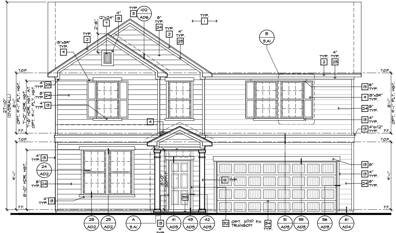
FRONT ELEVATION 'A' AT OPTIONAL 9'-1" PLT. HGT. SCALE 1/4"=1'-0" (22"X34") - 1/8"=1'-0" (11"X17")
