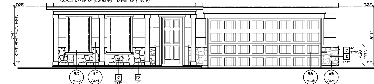
PARTIAL FRONT ELEVATION 'D' W/ STONE OPTION
