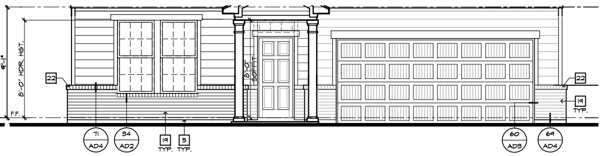
PARTIAL FRONT ELEVATION 'A' AT OPTIONAL 9'-1" PLT. HGT. W/ BRICK OPT. SCALE 1/4"=1'-0" (22"X34") - 1/8"=1'-0" (11"X17")
