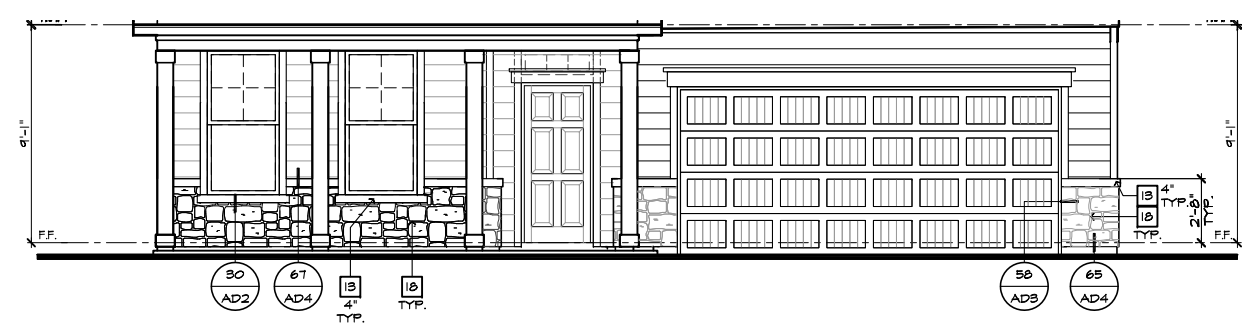
PARTIAL FRONT ELEVATION 'D' AT OPTIONAL 9'-1" PLT. HGT. W/ STONE OPT. SCALE 1/4"=1'-0" (22"X34") - 1/8"=1'-0" (11"X17")
