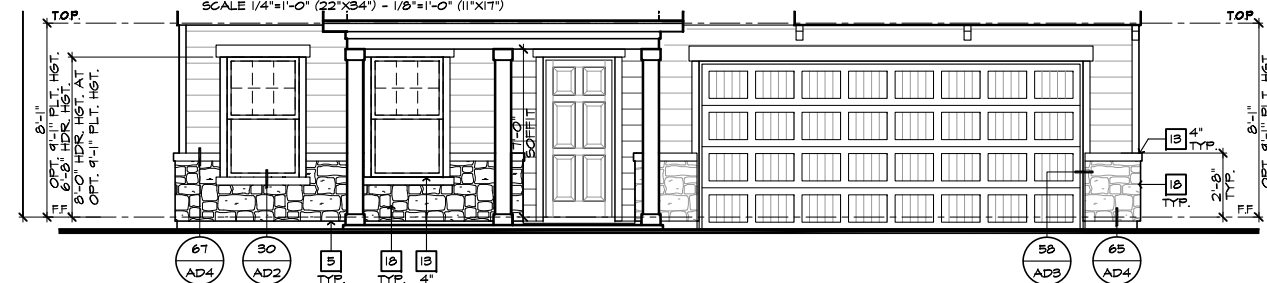
PARTIAL FRONT ELEVATION 'C' W/ STONE OPTION
