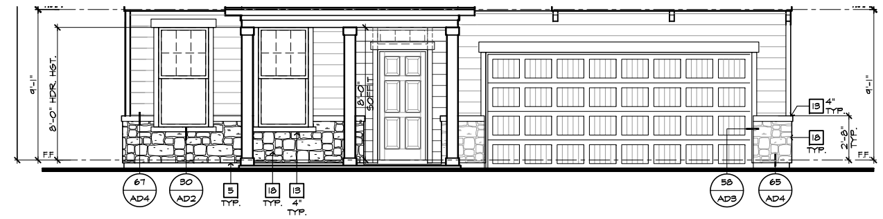
PARTIAL FRONT ELEVATION 'C' AT OPTIONAL 9'-1" PLT. HGT. W/ STONE OPT. SCALE 1/4"=1'-0" (22"X34") - 1/8"=1'-0" (11"X17")
