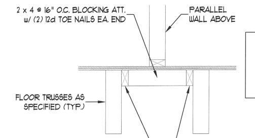
AN EXTRA TRUSS IS NOT REQUIRED WHEN FLOOR TRUSSES WITHIN THE NORMAL LAYOUT ARE POSITIONED BENEATH PARALLEL WALLS ABOVE. BY SEALING THE TRUSS DRAWINGS, THE ENGINEER OF RECORD FOR THE TRUSS SYSTEM ACKNOWLEDGES THE TRUSSES ARE DESIGNED FOR ALL IMPOSED LOADS INCLUDING THE ADDED DEAD LOAD OF THE WALL.
