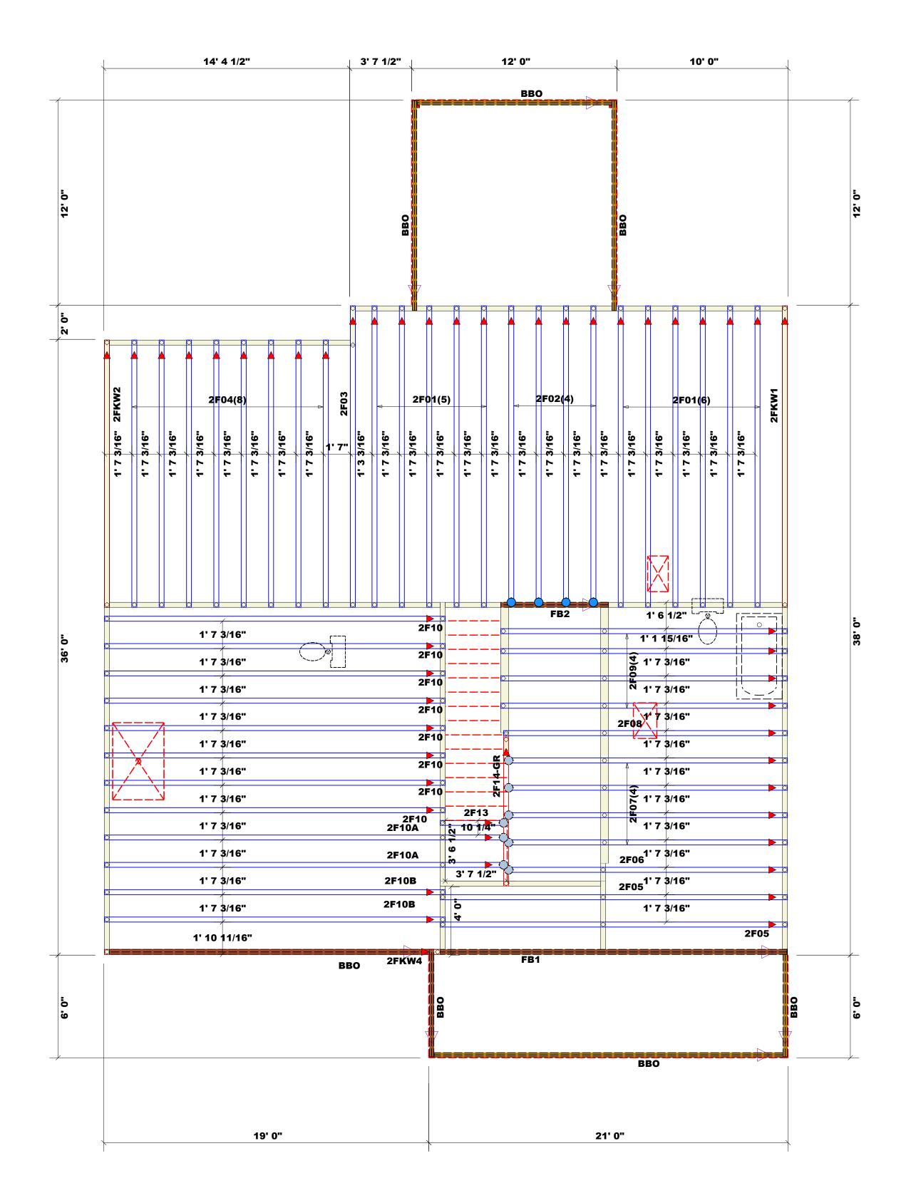
Truss Placement Plan SCALE: NTS
