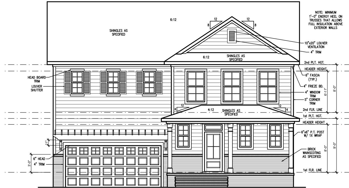
FRONT ELEVATION 'TRADITIONAL' (CRAWL/ STEM WALL ) SCALE: 1/4" = 1'-0" ON 22x34, 1/8" = 1'-0" ON 11x17 *SEE FOUNDATION PAGES FOR FOUNDATION TYPE
