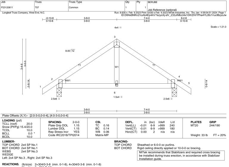
Max Horz 2=-76(LC 10) Max Uplift2=-61(LC 12), 4=-61(LC 12) Max Grav 2=373(LC 17), 4=373(LC 18)
