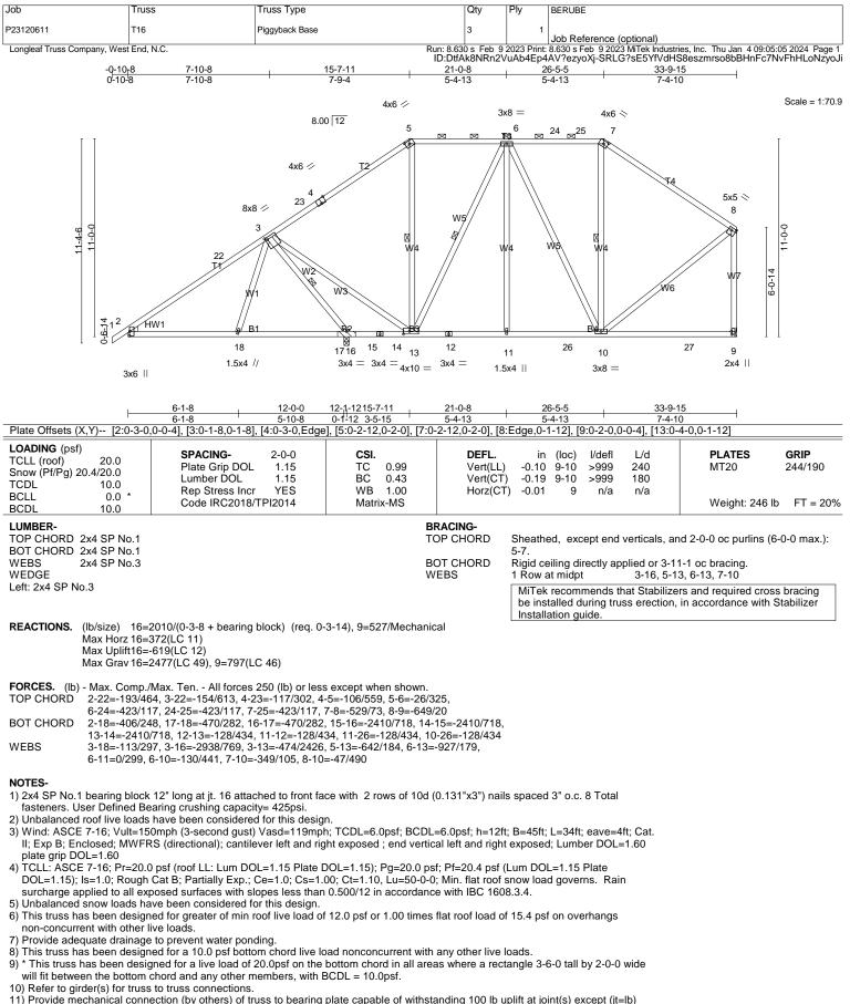
11) Provide mechanical connection (by others) of truss to bearing plate capable of withstanding 100 lb uplift at joint(s) except (jt=lb) 16=619.
