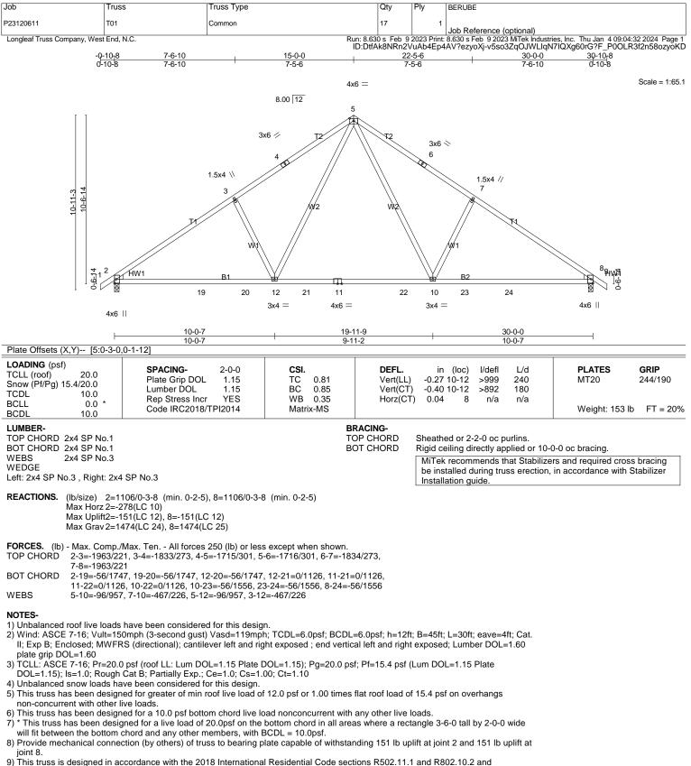
9) This truss is designed in accordance with the 2018 International Residential Code sections R502.11.1 and R802.10.2 and referenced standard ANSI/TPI 1.
