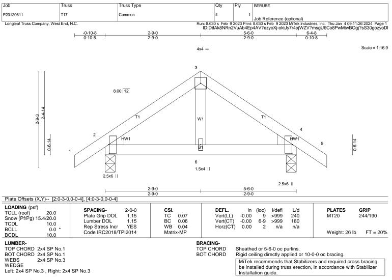
REACTIONS. (lb/size) 2=239/0-3-8 (min. 0-1-8), 4=239/0-3-8 (min. 0-1-8) Max Horz 2=-61(LC 10) Max Uplift2=-54(LC 12), 4=-54(LC 12) Max Grav 2=311(LC 17), 4=311(LC 18)
