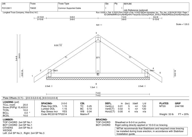
REACTIONS. (lb/size) 2=192/7-4-0 (min. 0-1-8), 4=192/7-4-0 (min. 0-1-8), 6=225/7-4-0 (min. 0-1-8) Max Horz 2=-76(LC 10) Max Uplift2=-75(LC 12), 4=-75(LC 12)
