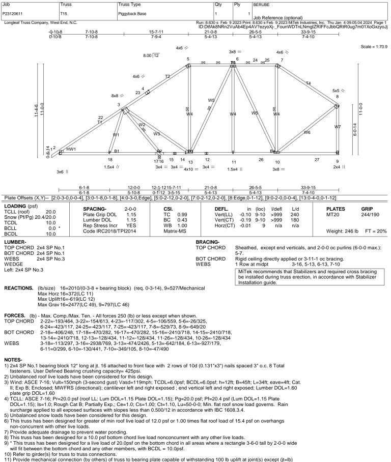
Provide mechanical connection (by others) of truss to bearing plate capable of withstanding 100 lb uplift at joint(s) except (jt=lb 16=619.
