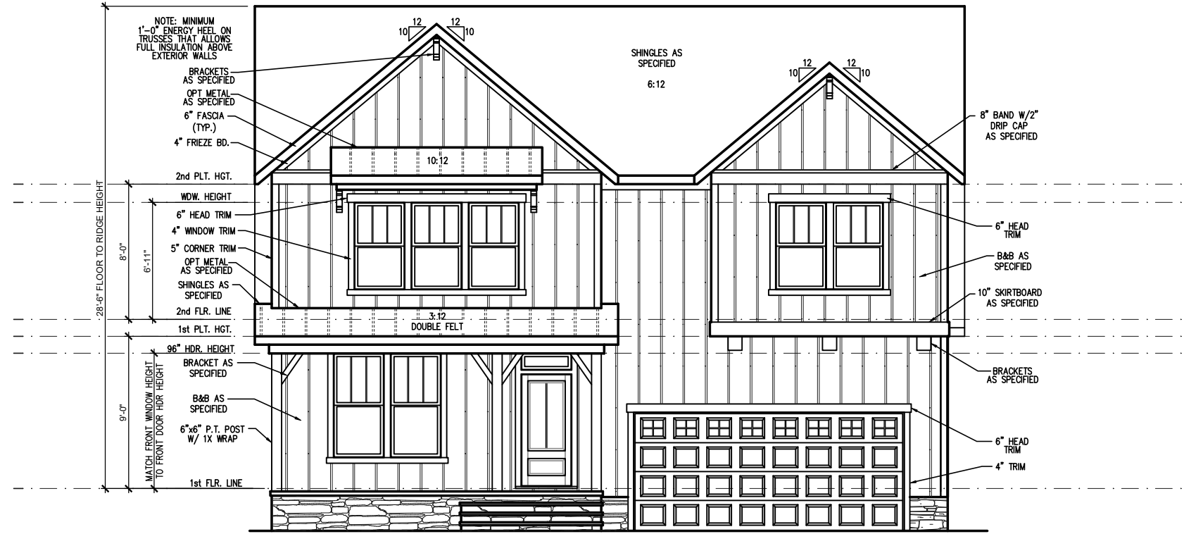
FRONT ELEVATION 'FARMHOUSE' (CRAWL/STEM WALL) SCALE: 1/4" = 1'-0" ON 22x34, 1/8" = 1'-0" ON 11x17 SEE FOUNDATION PAGE FOR FOUNDATION TYPE
