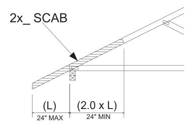
NOTE: TRUSS BUILT WITHOUT AN OVERHANG. THIS DETAIL IS NOT TO BE USED WHEN OVERHANG HAS BEEN BROKEN OFF.
