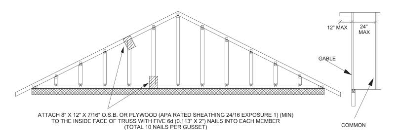
THE OUTSIDE FACE OF THE GABLE MUST BE SHEATHED WITH (MIN) 7/16" O.S.B OR PLYWOOD. SEE MITEK STANDARD GABLE END DETAILS FOR WIND BRACING REQUIREMENTS.
